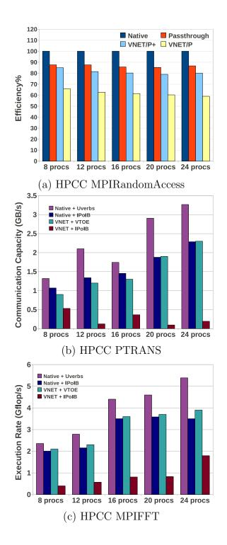
Figure 6.14: HPCC application benchmark results. VNET/P+ achieves near-native and scalable application performance when supporting parallel application workloads on 10 Gbps Ethernet with rigorous network communication.
