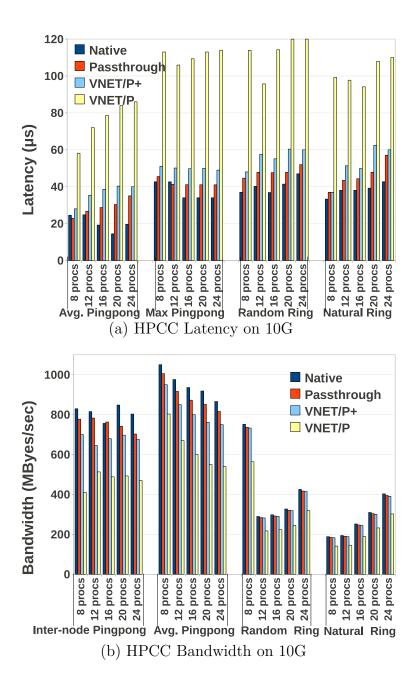
Figure 6.12: HPCC Latency-Bandwidth benchmark for all of Native, Passthrough VNET/P+, and VNET/P. The results are generally consistent with the previous microbenchmarks, while the ring-based tests show that latency and bandwidth of VNET/P+ scale and perform better than VNET/P.
