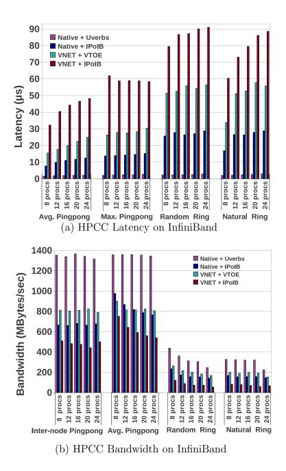
Figure 6.13: HPCC Latency-Bandwidth benchmark for all of Native+Uverb, Native+IPoIB, VNET+VTOE, and VNET+IPoIB. The results are generally consistent with the previous microbenchmarks, while the ring-based tests show that latency and bandwidth of VNET+VTOE scale and perform better than VNET+IPoIB.
