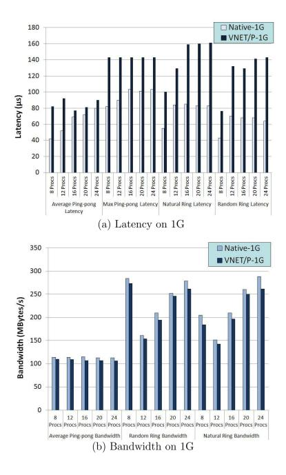
Figure 6.11: HPCC Latency-bandwidth benchmark for 1 Gbps Ethernet. Ring-based bandwidths are multiplied by the total number of processes in the test. The pingpong latency and bandwidth tests show results that are consistent with the previous microbenchmarks, while the ring-based tests show that latency and bandwidth of VNET/P scale similarly to the native cases.
