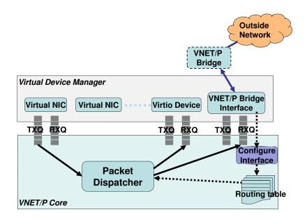
Figure 5.2: VNET/P core's internal logic.
