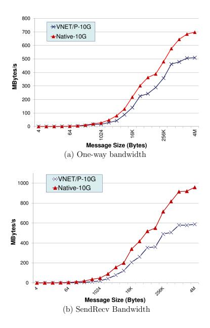
Figure 6.8: Intel MPI PingPong microbenchmark showing (a) one-way bandwidth and (b) bidirectional bandwidth as a function of message size on the 10 Gbps hardware.
