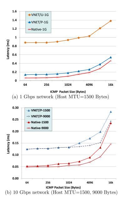
Figure 6.2: End-to-end round-trip latency of VNET/P as a function of ICMP packet size. Small packet latencies on a 10 Gbps network in VNET/P are  $\sim$ 130  $\mu$ s.
