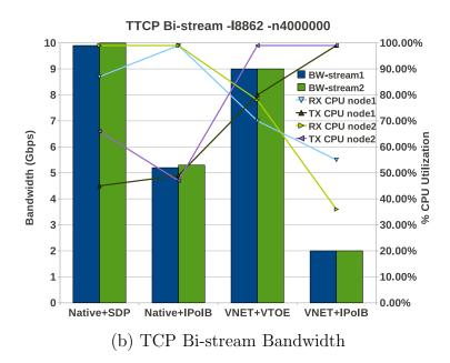
Figure 6.4: End-to-end TCP throughput and CPU utilization of Native+SDP, Native+IPoIB, VNET+VTOE, and VNET+IPoIB on InfiniBand Interconnect. VNET+VTOE performs more than 2.5 times better then VNET+IPoIB on the InfiniBand Interconnect
