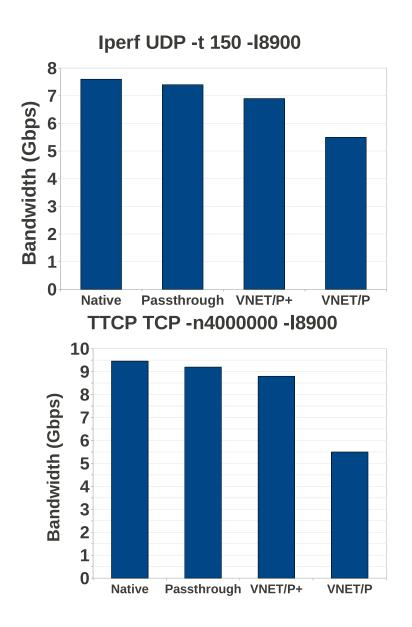
Figure 6.3: End-to-end UDP goodput and TCP throughput of VNET/P+ and VNET/P on 10 Gbps network. VNET/P+ performs better then VNET/P for the 10 Gbps network
