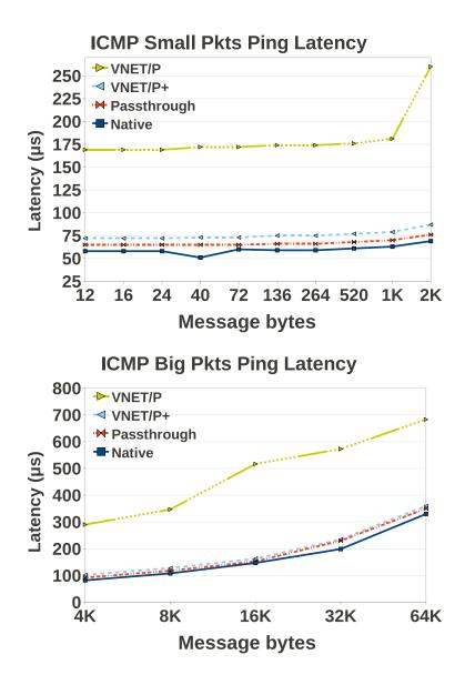
Figure 6.5: End-to-end round-trip latency of VNET as a function of ICMP packet size. Small packet latencies are: VNET/P+— $72\mu$ s, Passthrough— $65\mu$ s, Native— $58\mu$ s, VNET/P— $169\mu$ s.
