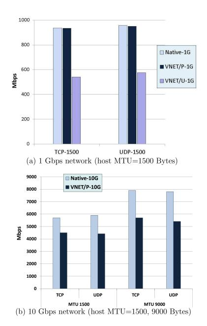
Figure 6.1: End-to-end TCP throughput and UDP goodput of VNET/P on 1 Gbps network. VNET/P performs identically to the native case for the 1 Gbps network and achieves 74–78% of native throughput for the 10 Gbps network.
