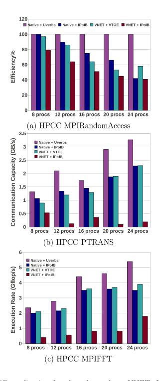
Figure 6.15: HPCC application benchmark results. VNET+VTOE approaches Native+IPoIB performance and scalable application performance when supporting parallel application workloads on InfiniBand with rigorous network communication.
