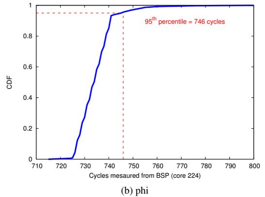
Figure 5: CDF of IPI one-way latencies, the hardware limit of asynchronous signaling that is available to HRTs.
