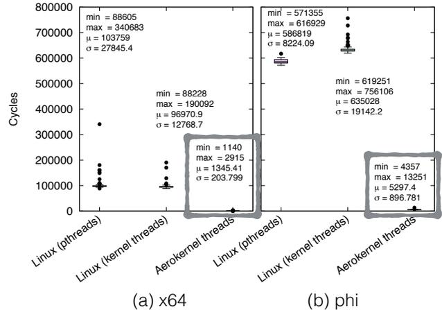
Figure 2: Thread creation latency. Aerokernel thread creations are on average two orders of magnitude faster than Linux userspace (pthreads) or kernel thread creations and have at least an order of magnitude lower variance.
